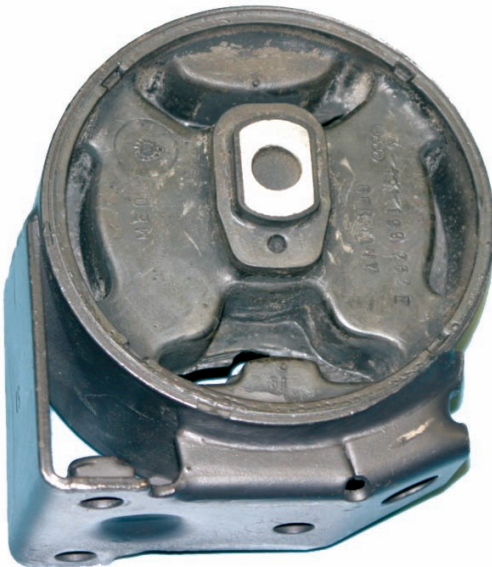
Figure 2-1. Engine mount of a Volkswagen Golf II, 1985.
